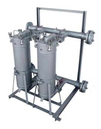
Standard material of construction for the Top Entry MultiPlex WP series bag filter housing is wetted 316 stainless steel. The filter's lid assembly is an investment casting of the same material. The leg skid assembly and bolting are painted or plated carbon steel. Standard o-ring material is Viton in both front and rear seals. The standard drain port for each vessel is 3/4" FNPT, mounted in the bottom of the elliptical head.
