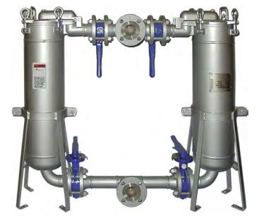
The standard material used for construction of the Top Entry DuPlex bag housing is 316 stainless steel for all wetted parts. The housing lid assembly is an investment casting of the same material. The leg assembly is plated carbon steel and painted. The standard drain port for each vessel is 3/4" FNPT, mounted in the bottom elliptical head. There are two 1/4" FNPT vent/gauge ports located at the top of the lid assembly, as well as on the inlet and outlet manifold.
