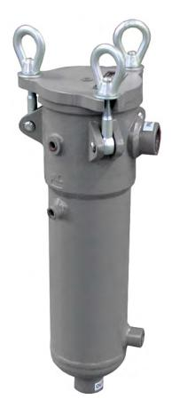
W4 series bag filter housings are designed for operation to 300 psi or optional design pressures to 500 psi. These housings have a large sump area at the bottom of the basket for particulate accumulation. This design utilizes the filter more efficiently and prolongs the life of the bag filter.
