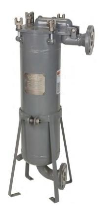
The standard material of construction for the W8T series top entry single bag housing is 316 Stainless Steel. The closure lid assembly is an investment casting of the same material. The leg assembly and bolting are painted or plated carbon steel. Standard o-ring material is Viton in both front and rear seals. The standard drain port is 3/4 inch FNPT, which is mounted in the bottom of the elliptical. There are two 1/4 inch FNPT vent/gauge ports located at the top of the lid assembly.
